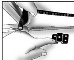
C. Pre-drill the mounting holes using a 7/64" drill bit.
