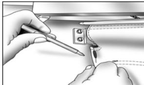
C. Mark the fastener mounting holes and pre-drill each hole using a 7/64" drill bit.
