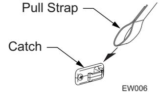
**CAUTION** Do not release the strap until the awning is against the coach wall. Releasing the strap early will cause the awning to slam against the wall causing damage to the awning and/or vehicle.
