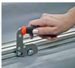
Cut fabric using the rotating cutting blade.
