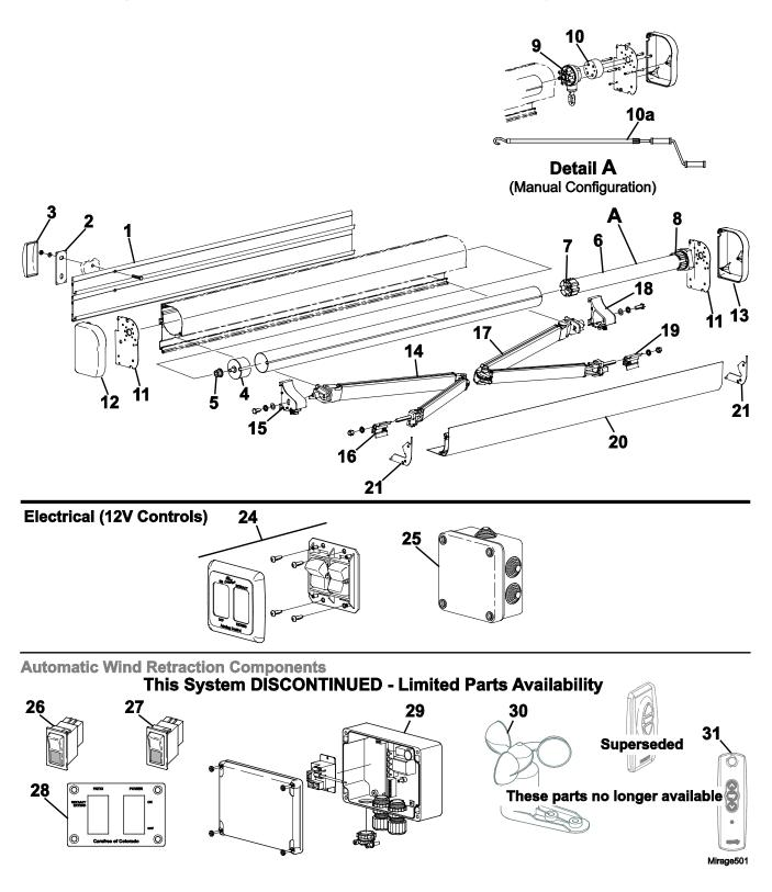
Electronic components shown are not used for the Direct Response system. For Direct Response Electronics, Refer to "ELECTRONIC SYSTEMS AND COMPONENTS"
