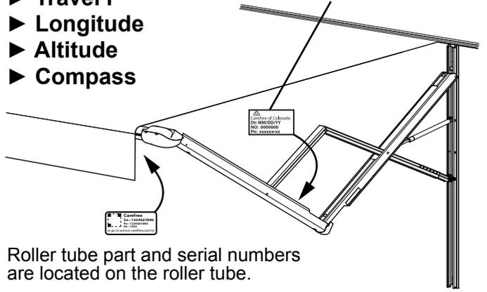
Roller tube part and serial numbers are located on the roller tube.
