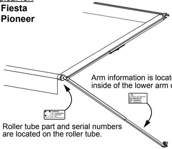
Roller tube part and serial numbers are located on the roller tube.
